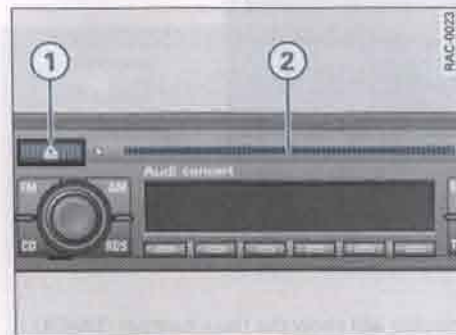
Fig. 24 CD eject button and CD slot
